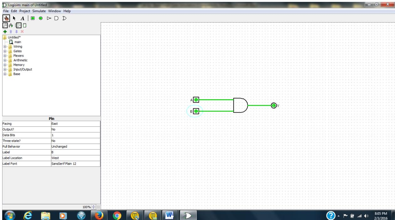
Figure 6. Logisim: Verifying the AND gate through Simulation.
