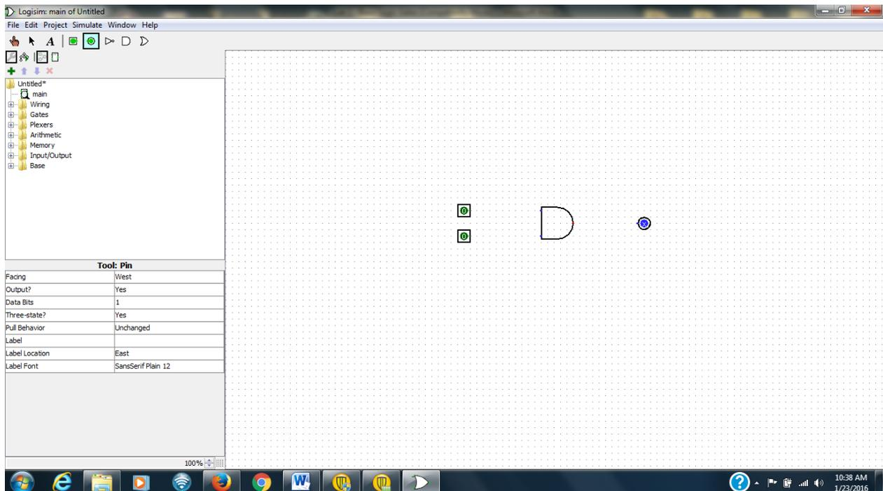
Figure 3. Logisim: Placing Inputs and Outputs.
