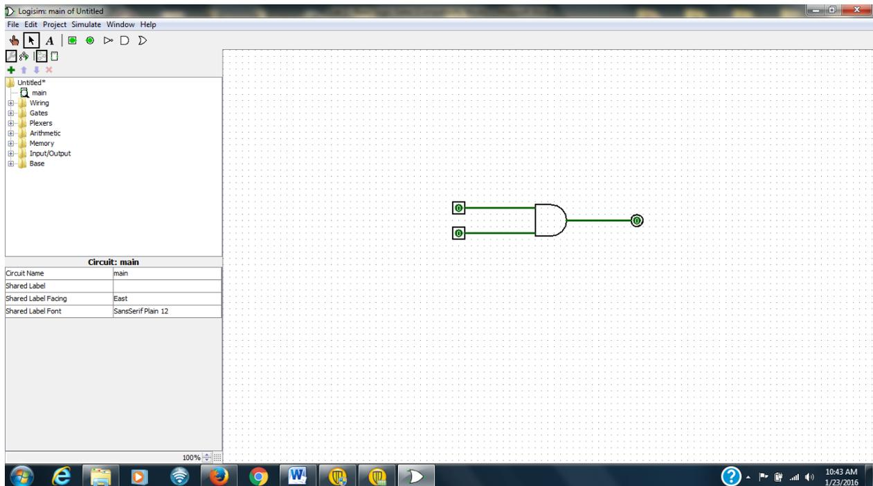
Figure 4. Logisim: Placing Wires.
