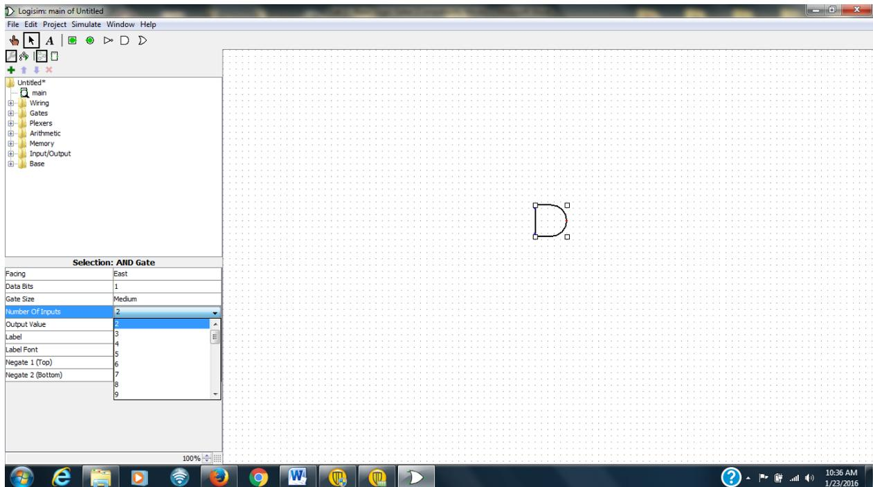
Figure 2. Logisim: Placing an AND Gate.
